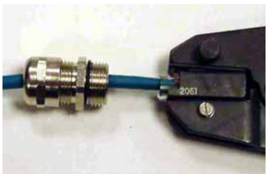
Step 4: Insert conductors and crimp
