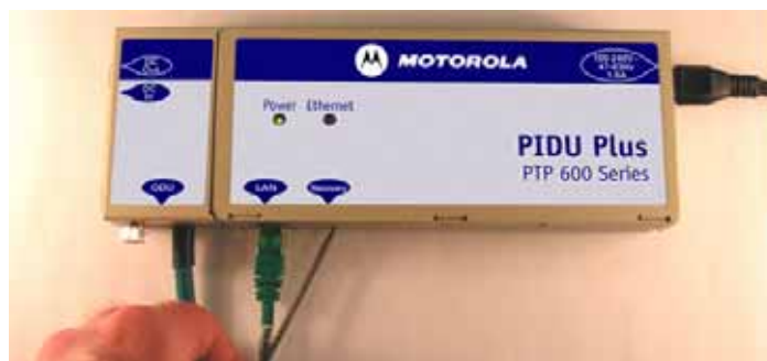
Figure 5 – PIDU Plus Recovery Switch Location
