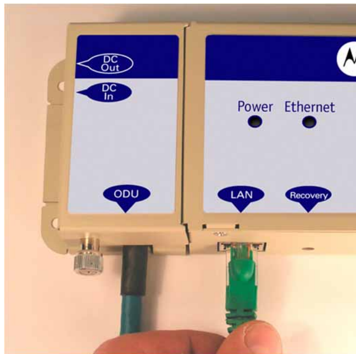
Figure 31 - Making the Network Connection at the PIDU Plus
