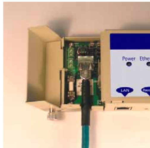
Step 2: Plug in the ODU into the PIDU Plus Cable ensuring that it snaps home
