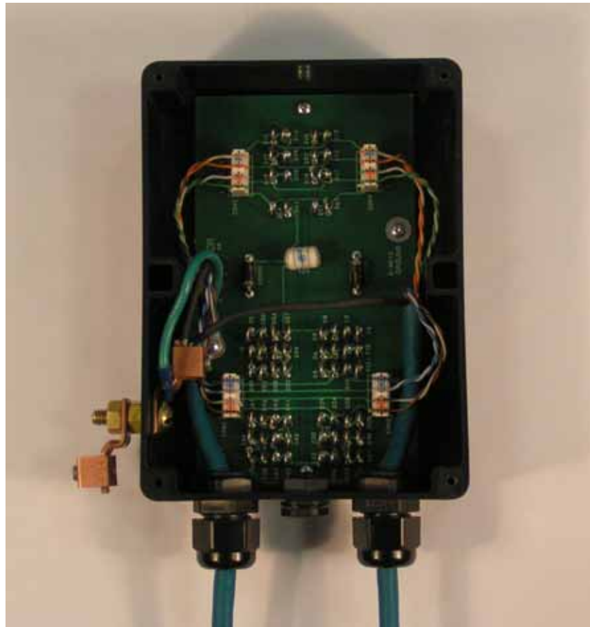
Figure 112 - Surge Arrester ALPU-ORT Connection Illustration
