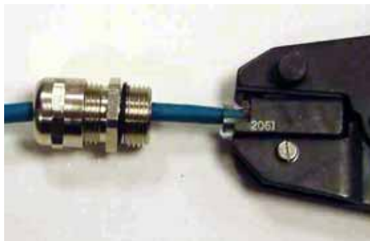
Step 4: Insert conductors and crimp
