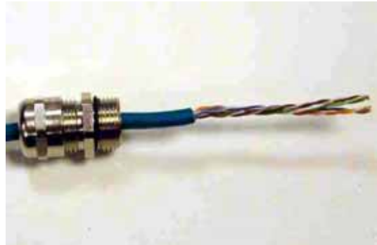
Step 2: Strip the outer insulation
