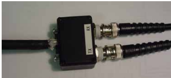
Figure 141 - Example of a Balun
