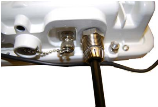
Step 3: Screw in the body of the weather proofing gland and tighten
