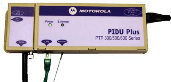
Figure 4 – PIDU Plus Recovery Switch Location
