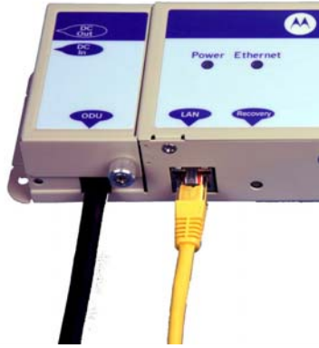
Figure 22 - Making the Network Connection at the PIDU Plus
