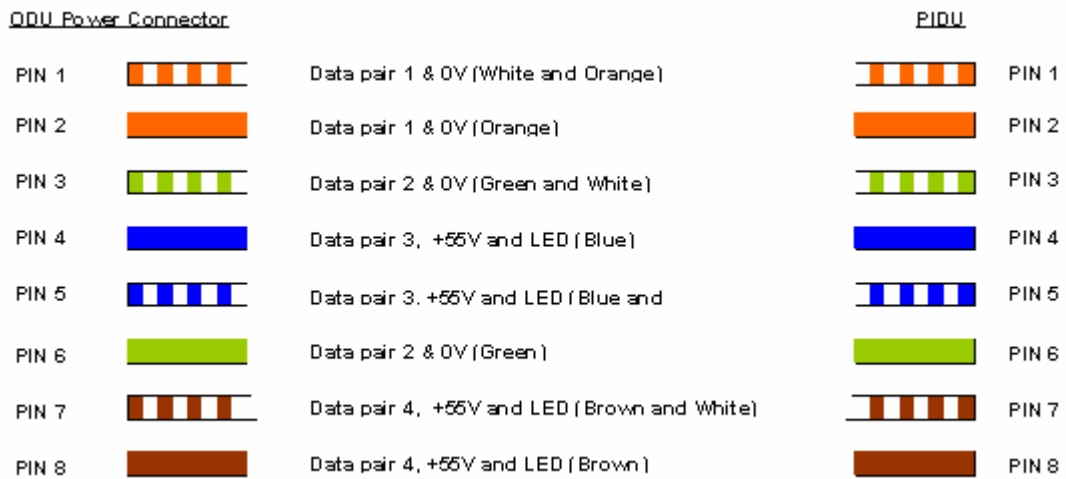
Figure 126 - Cable Connection Diagram (T568B Color Coding)
