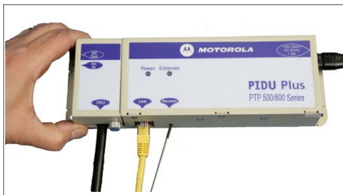
Figure 4 PIDU Plus Recovery Switch Location
