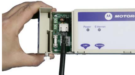
Step 2: Plug in the ODU into the PIDU Plus Cable ensuring that it snaps home
