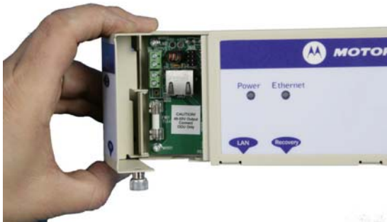
Step 1: Undo the retaining screw and hinge back the cover
