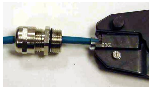
Step 4: Insert conductors and crimp
