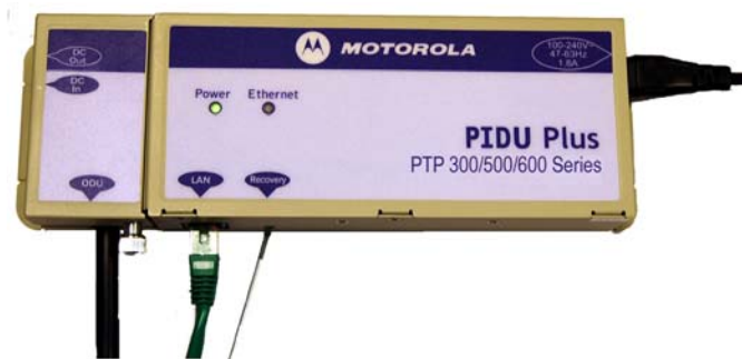
Figure 1-5 PIDU Plus recovery switch location
