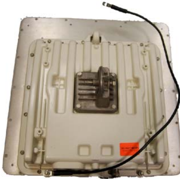
Figure 18 – ODU with Mounting Bracket and Earth Bonding Lead
