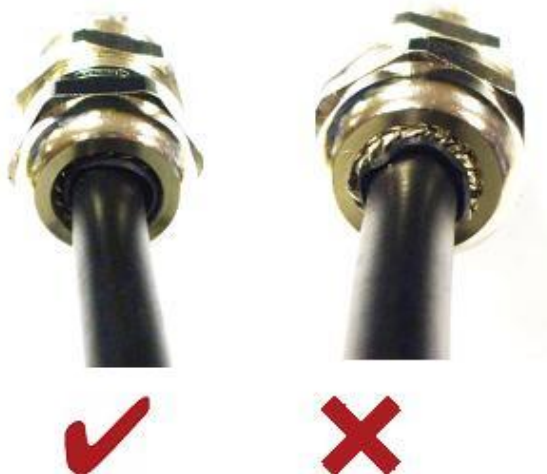
Figure 25 - Correct and Incorrect Tightening of Cable Gland
