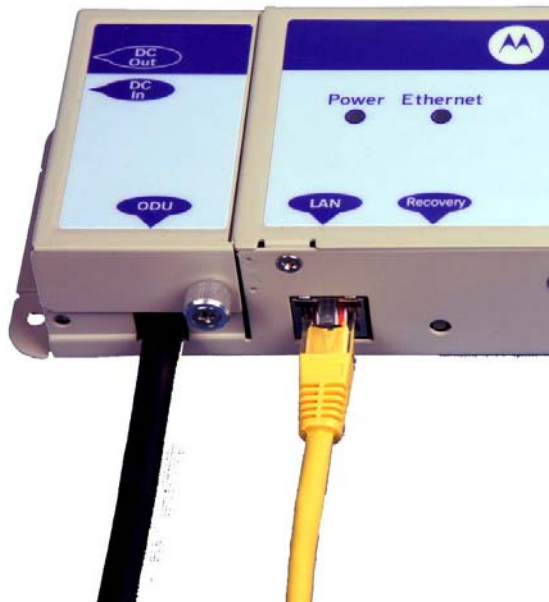
Figure 30 - Making the Network Connection at the PIDU Plus
