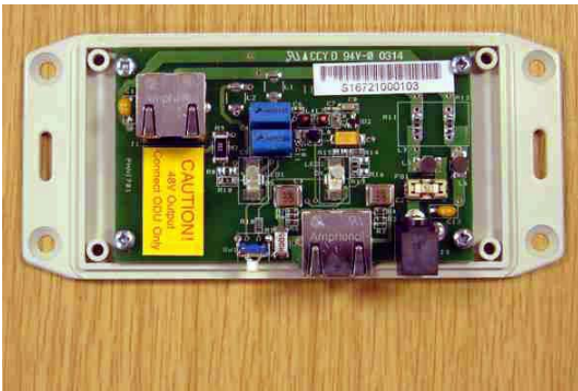
Step 1: Remove the cover by removing the four cover fixing screws.
