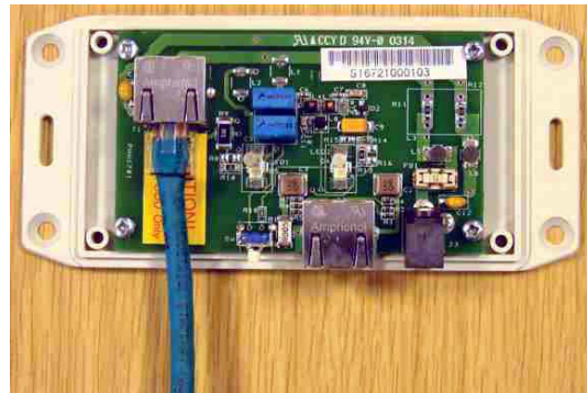
Step 2: Plug in the ODU to IDU Cable ensuring that it snaps home
