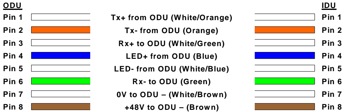
Figure 33 ODU to IDU Connection Diagram
