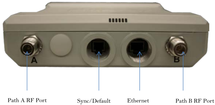
Figure 4 AP interfaces – 2.4 GHz, 3.5 GHz, 3.6GHz, 5 GHz
