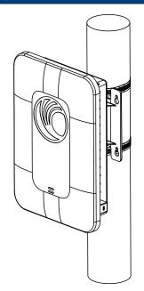
Attach the cnPilot E500 to the mounting bracket.
