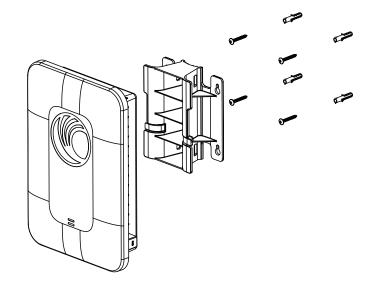
Insert the wall anchors into the wall using the mounting bracket as a template and insert the screws.
