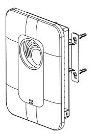
Attach the cnPilot E500 to the mounting bracket.
