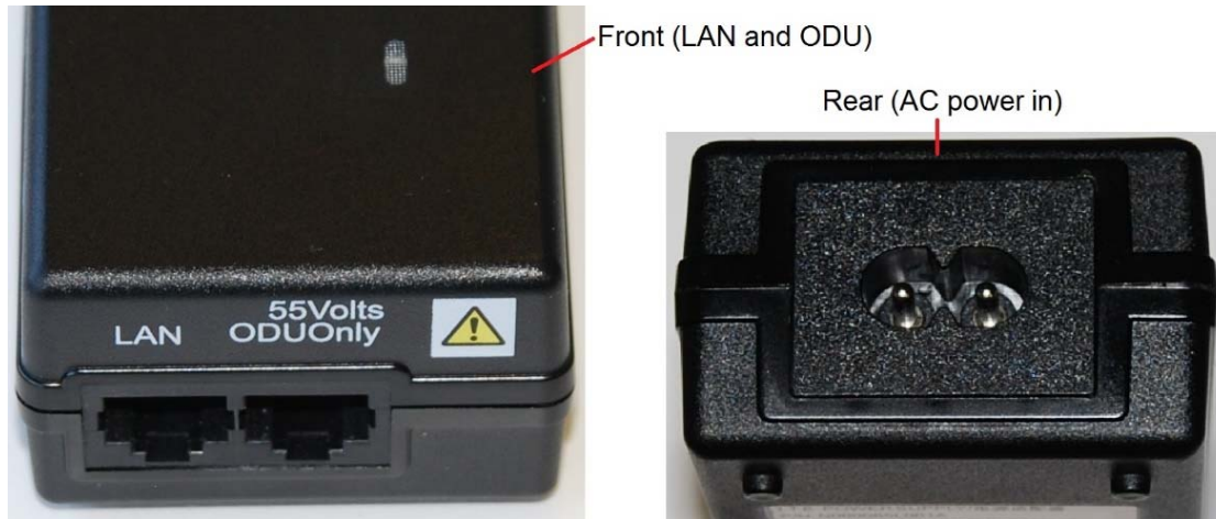
Figure 11 AC Power Injector interfaces
