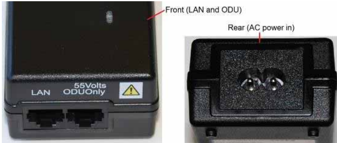
Figure 15 AC Power Injector interfaces
