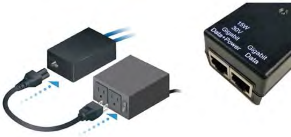
Figure 33 : Installation of adapter to power outlet
