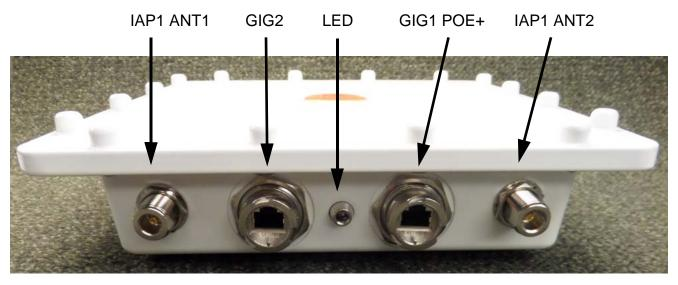
The XH2-120 has four male Type N connectors for the antennas.
