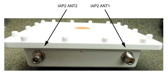
Both of the AP's RADIO1 cables (RADIO1 ANT1 and RADIO1 ANT2) must be attached to antenna leads for the same frequency band (for example, 2.4GHz), and RADIO1 must be set to that band on the AP (see Step 10). Similarly, both RADIO2 cables need to go to the same frequency band on the antenna (for example, 5GHz). For simplicity, if you are using an antenna with two 2.4GHz leads and two 5GHz leads, we suggest that you connect RADIO1 (ANT1 and
