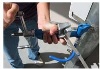
Once the strap is satisfactorily tight, rotate the Band-It tool back so that the strap cannot slide back through the buckle.
