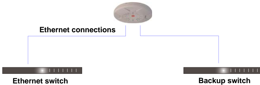
Figure 24. Switch Failover Protection
