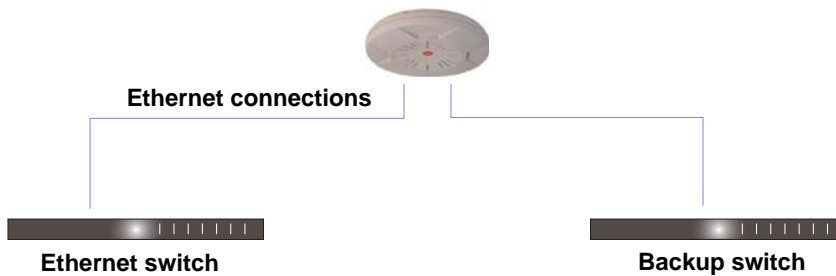
Figure 24. Switch Failover Protection
