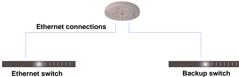
Figure 26. Switch Failover Protection
