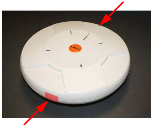
Figure 191. Tamper-evident seal locations for XN4 indicated by arrows
