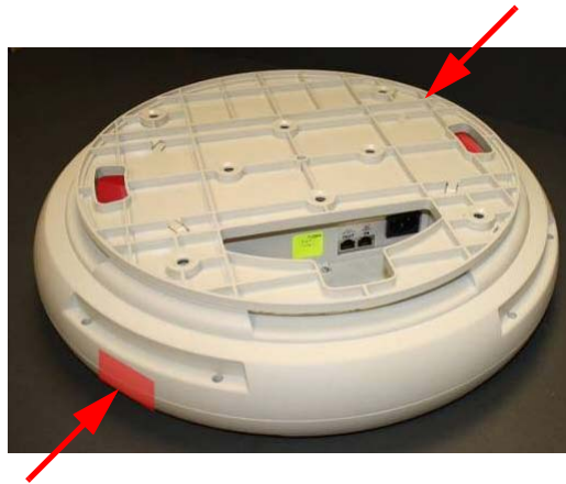
Figure 192. Two tamper-evident seals on seam of XN8/12/16
