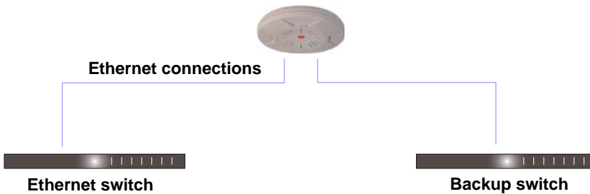
Figure 27. Switch Failover Protection
