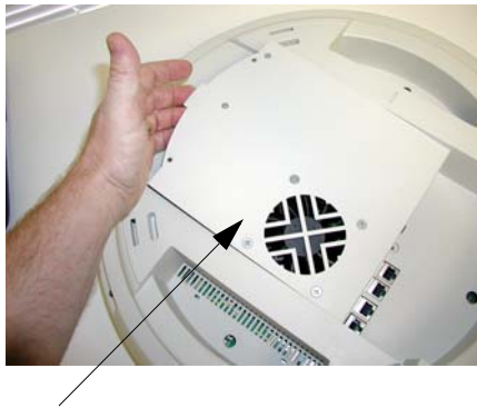
Access panel (with power supply and fan)
