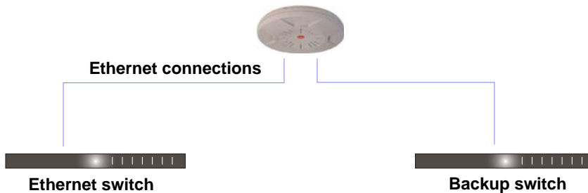
Figure 30. Switch Failover Protection
