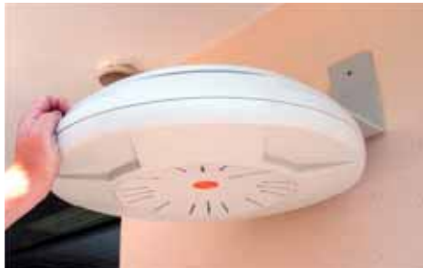
Figure 50. Mounting the Array on a Wall
