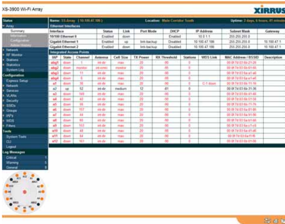
Figure 6. WMI: Array Status
