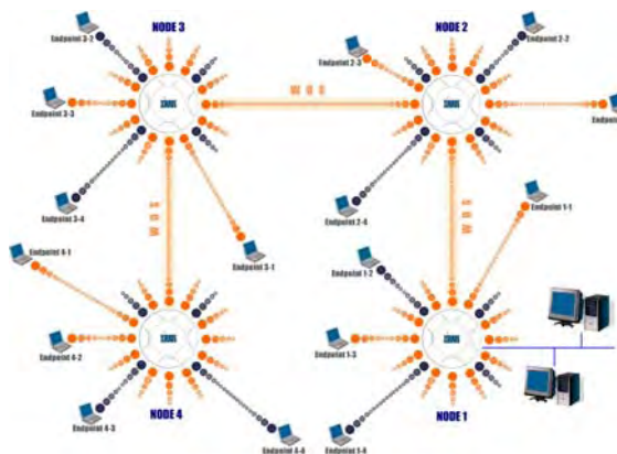
Figure 23. A Multiple Hop WDS Connection
