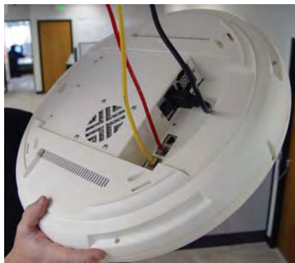
Figure 30. Connecting the Cables
