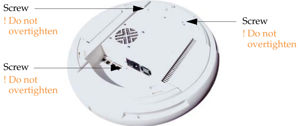
Figure 179. Reinstalling the Access Panel
