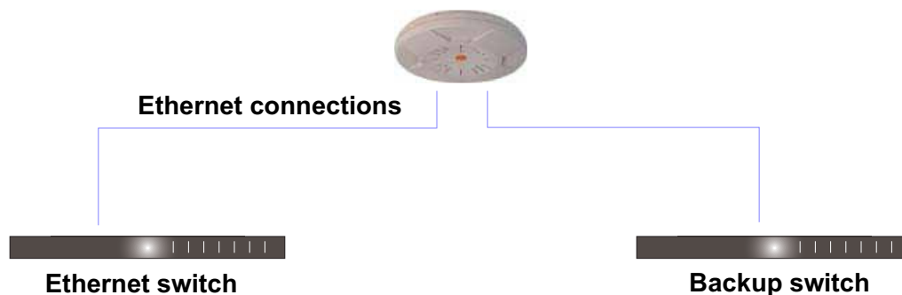
Figure 30. Switch Failover Protection
