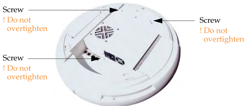
Figure 159. Reinstalling the Access Panel
