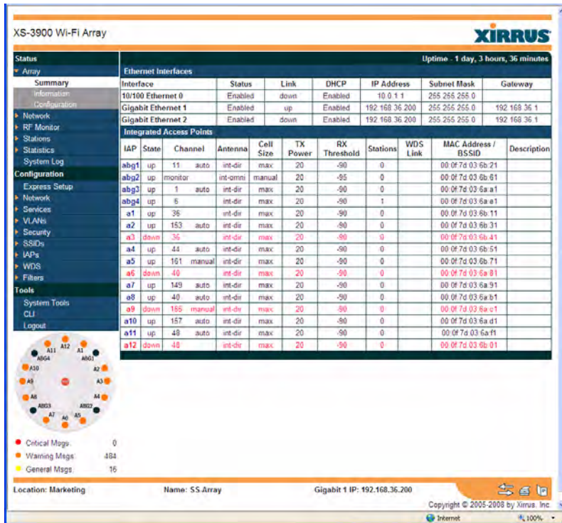
Figure 5. WMI: Array Status
