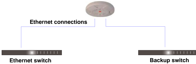
Figure 21. Switch Failover Protection
