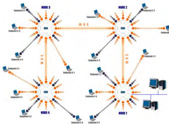
Figure 23. A Multiple Hop WDS Connection
