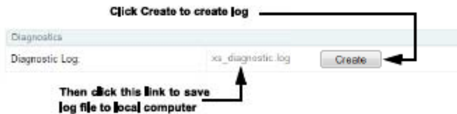
Figure 176. Saving the Diagnostic Log
