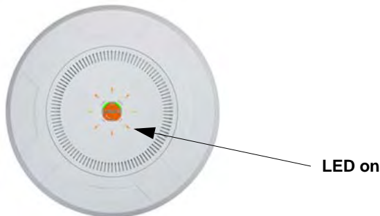
Figure 97. LEDs are Switched On
