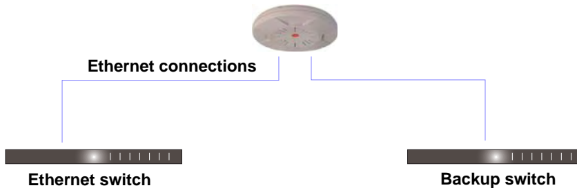
Figure 23. Switch Failover Protection
