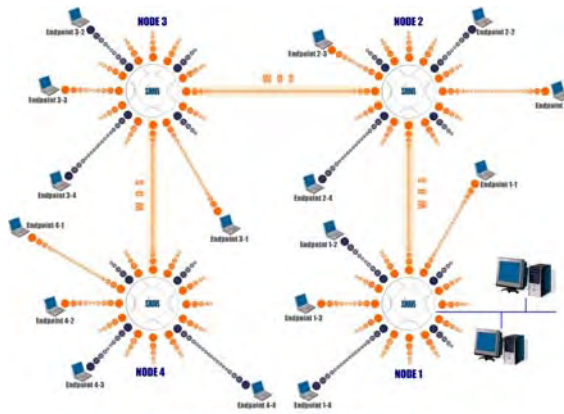
Figure 26. A Multiple Hop WDS Connection
