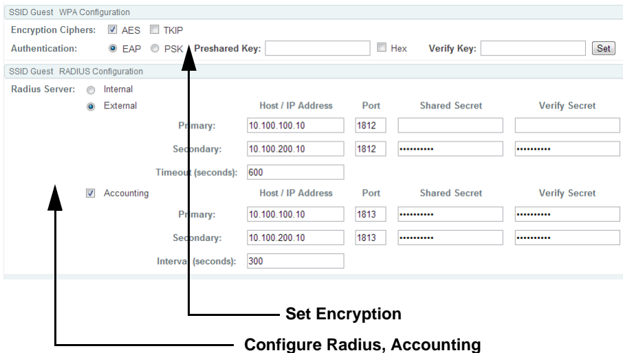
Figure 139. SSID Management—Encryption, Authentication, Accounting
