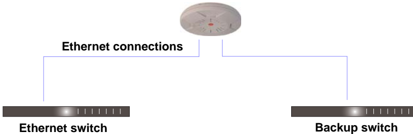
Figure 23. Switch Failover Protection
