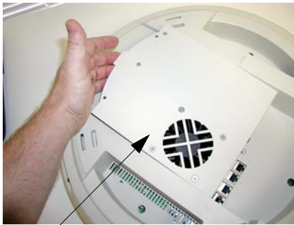
Access panel (with power supply and fan)
