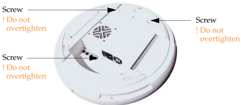
Figure 115. Reinstalling the Access Panel
