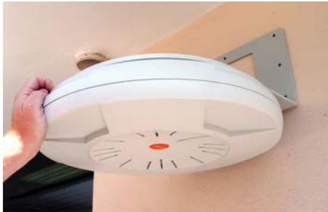
Figure 42. Mounting the Array on a Wall
