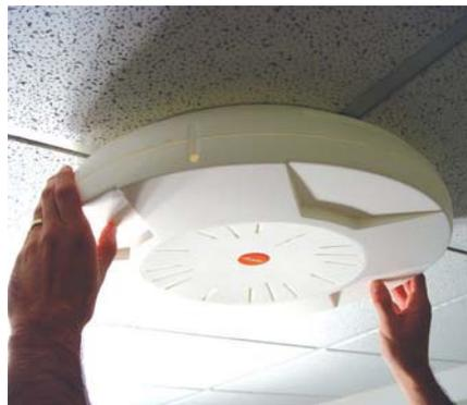
Figure 28. Attaching the Unit (XS-3900)
