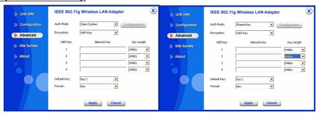
**WEP Key 1~4**: choose the encryption way, either in HEX or ASCII formats, and enter the password in the blank space.
