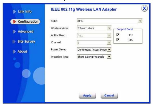
**SSID:** Service Set Identifier, which is a unique name shared among all clients and nodes in a wireless network. The SSID must be identical for each clients and nodes in the wireless network.
