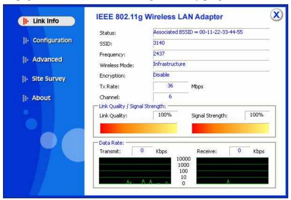
**Status:** Shows the BSSID associated, which can be used to identify the wireless network.
