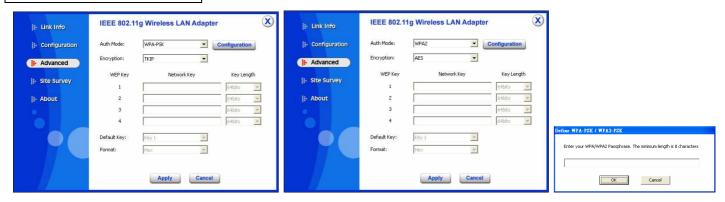
If WPA-PSK or WPA2-PSK is selected, the above screen is shown. Please select the encryption type from drop down menu and press *Configuration* button to configure the passphrase key.
