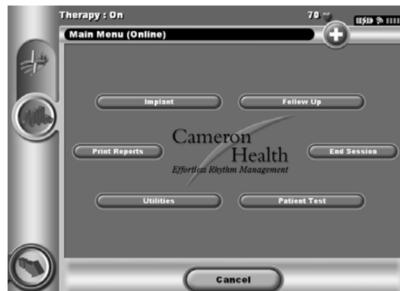
Figure 34: Select the Patient Test Button to access the Manual Shock Test screen.
