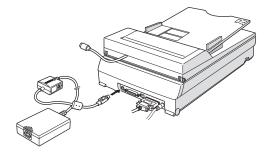
2. Slide the cover on the connector block so that the ADF connector is visible.
