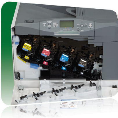
Front-load access to toner cartridges on LBP5460
