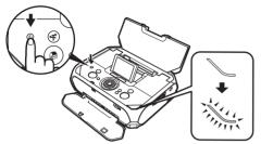
The Power lamp flashes, then changes to steady (non-flashing).
