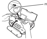
(1) Slide the Lock Switch toward the right to open the Printer Cover.
