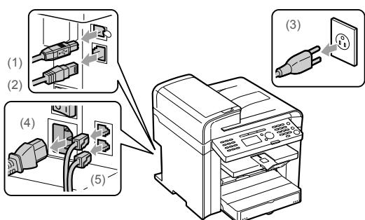
How to remove the cables and cord
