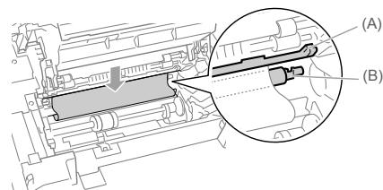
(2) When the leading edge emerges, hold both sides of the jammed paper and carefully pull it out.
