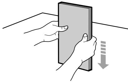
(5) Gently load the envelopes into the paper cassette with the print side face up, until the edge of the envelope stack meets the back of the paper cassette.
