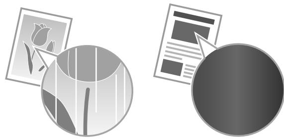
\* No message appears on the display even if the toner almost runs out. Replace the toner cartridge when white streaks appear on the printouts or some parts of the printout are faded.
