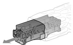
Shake the toner cartridge 5 or 6 times as shown in the figure to evenly distribute the toner inside the cartridge.
