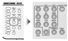
Press [O] (Coded Dial), and then enter the three-digit registration number (001 to 181) with the numeric keys.
