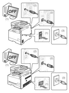
When installing and removing the optional accessories, be sure to turn the machine off, unplug the power plug, and then disconnect all the interface cables and power cord from the machine. Otherwise, the power cord or interface cables may be damaged, resulting in a fire or electrical shock.
