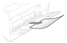
**If the jammed paper cannot be removed easily**Do not try to remove it forcefully but proceed to Step 3.
