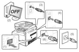
How to remove the cables and cord
