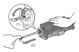
Remove the drum protective cover (A).
