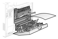
6 Holding the tabs (A) on both sides, close the duplex unit.
