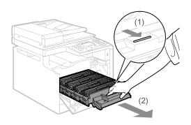
3 Hold the toner cartridge to be replaced by its handle and pull it straight up and out of the machine.
