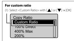
(2) Specify the ratio with  $[\blacktriangle]$  or  $[\blacktriangledown] \rightarrow [OK]$ You can also enter the copy ratio using the numeric keys. **Custom Ratio** 100 |% (25-400)
