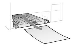
**If the jammed paper cannot be removed easily** Do not try to remove it forcefully but proceed to Step 7.
