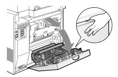
**3** Open the paper output guide by holding the green tab (A).
