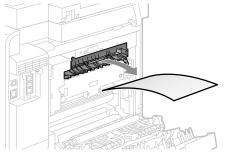
Make sure that no paper is jammed inside the paper output guide, and then close it.
