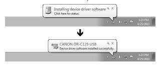
When the scanner is properly connected to the computer, the (CaptureOnTouch) icon appears on the taskbar (or menu bar) as follows.
