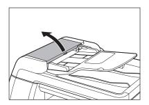
Clean the rollers and rubber parts (A) inside the ADF cover with a cloth dampened with water. Then wipe the area with a soft, dry cloth.
