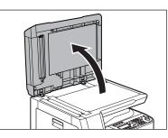
Clean the platen glass and the underside of the ADF/platen glass cover with a cloth dampened with water. Then wipe the area with a soft, dry cloth.
