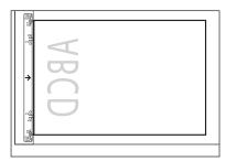
If your original does not match any of the paper size marks, align the center of your original with the arrow mark.
