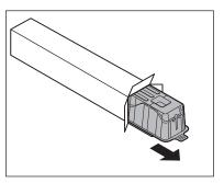
Open the case and remove the toner cartridge. Keep the box and case for future use.
