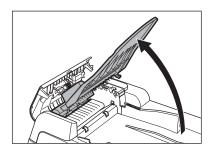
Clean the rollers (B) below the document feeder tray with a cloth dampened with water. Then wipe the area with a soft, dry cloth.
