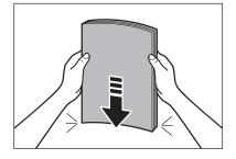
Load the paper stack of the appropriate size with the print side facing up.
