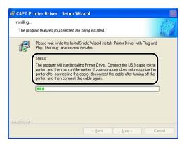
Connect the printer to the computer with the USB cable.
