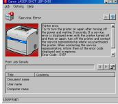
If the error has appeared, cycle the power of the printer using the following procedure. The service error message may disappear.
