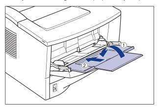
Be sure to return the extension tray to its original position. To avoid damaging the multi-purpose tray, do not close the multi-purpose tray with the extension tray left open.
