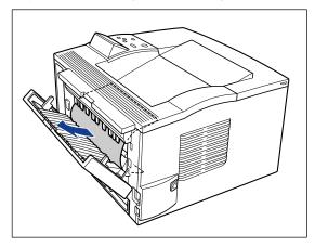
When you are having trouble removing the jammed paper from the printer, slightly tilt the sub-output tray ① as shown in the illustration below, and remove the pins from the hooks on right and left sides of the tray ②.
