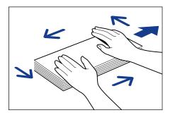
Flex the stack on all four sides to remove any stiffness as illustrated below. If the corners are curled, straighten them.
