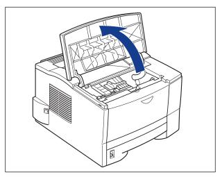
Re-install the toner cartridge in the printer.
