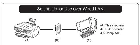
When the machine has not been connected to the network, perform this setup to use the machine over wired LAN. This setup procedure requires settings to be performed on the machine and the computer.
