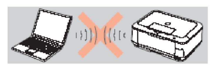
An "Ad-hoc connection," which establishes a direct connection to the computer over a wireless connection without using an access point, is not supported.
