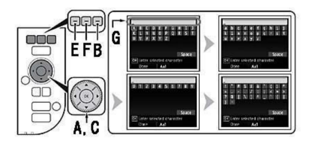
1. When the on-screen keyboard shown above is displayed, press the center FUNCTION button (A) to switch to a keyboard having the characters you want to use.
