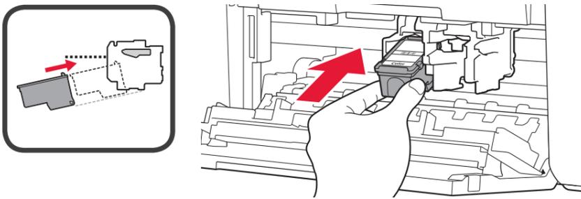
4 EN Push the FINE Cartridge in and up firmly until it snaps into place.
