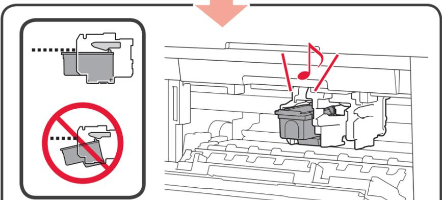
EN A beep sounds when the FINE Cartridge is installed correctly.
