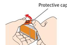
**NOTE:** To avoid spilling ink, never press on the sides of an ink tank.
