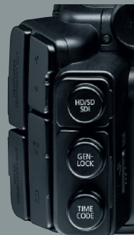
BNC style HD-SDI, Genlock, Time Code input and output terminals (XH G1S)
